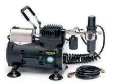
Iwata Smart Jet airbrush compressor is compact and quiet, producing a preset working pressure of 20-25 PSI. It is a good choice for general purpose applications that require low to medium air pressure.
